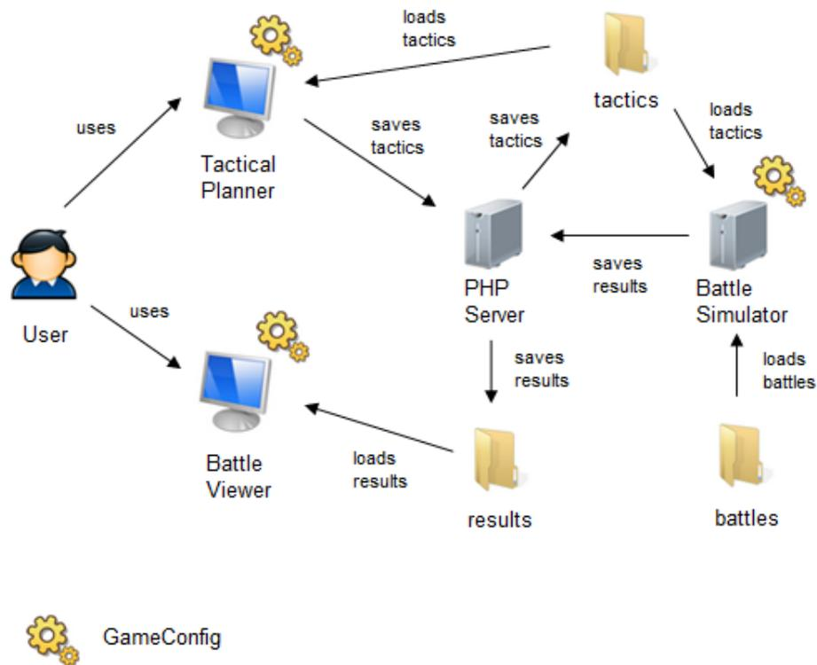
**Figure 2 - The Platform architecture**
