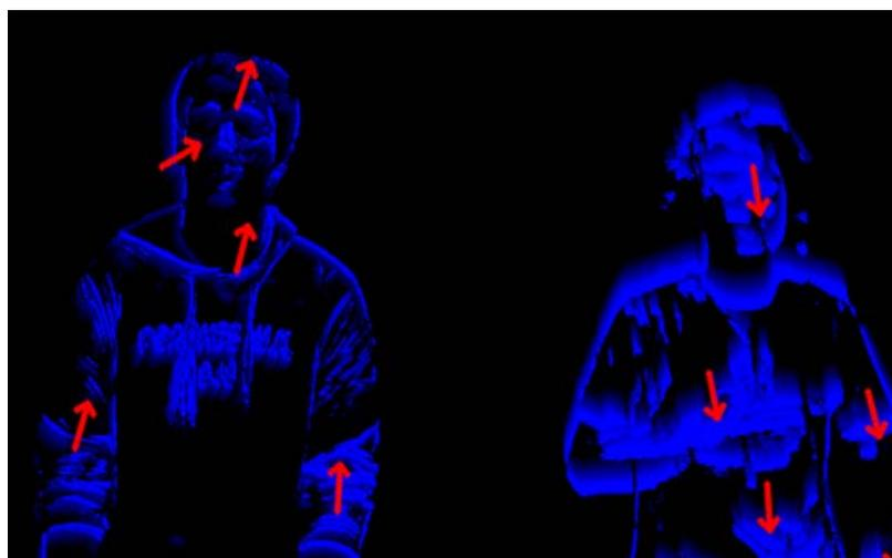
Figure 9: Motion vectors detected, based on optical flow extraction from an image sequence.
