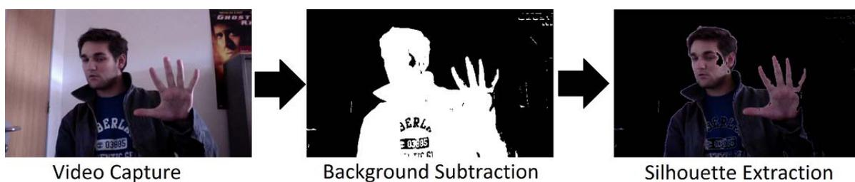
Figure 8: Silhouette extraction pipeline
